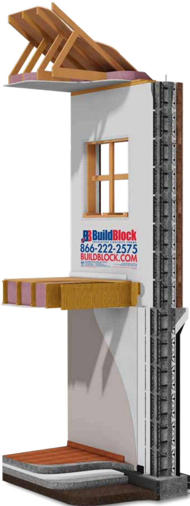
**CAUTION:** When installing a waterproofing membrane, ensure the membrane is mechanically attached using a thin furring strip of wood or metal at the very top of the wall above the final finish grade by 8" to 12".
