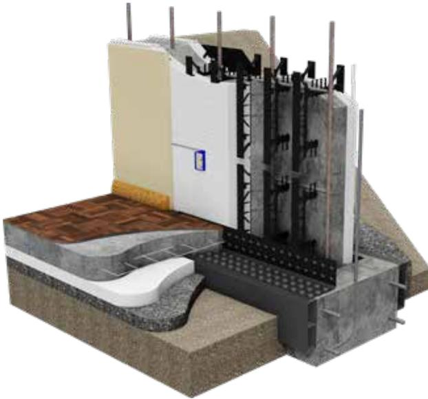
Additional interior waterproofing system using CactusBoard, Form-a-Drain, and appropriate backfill.
