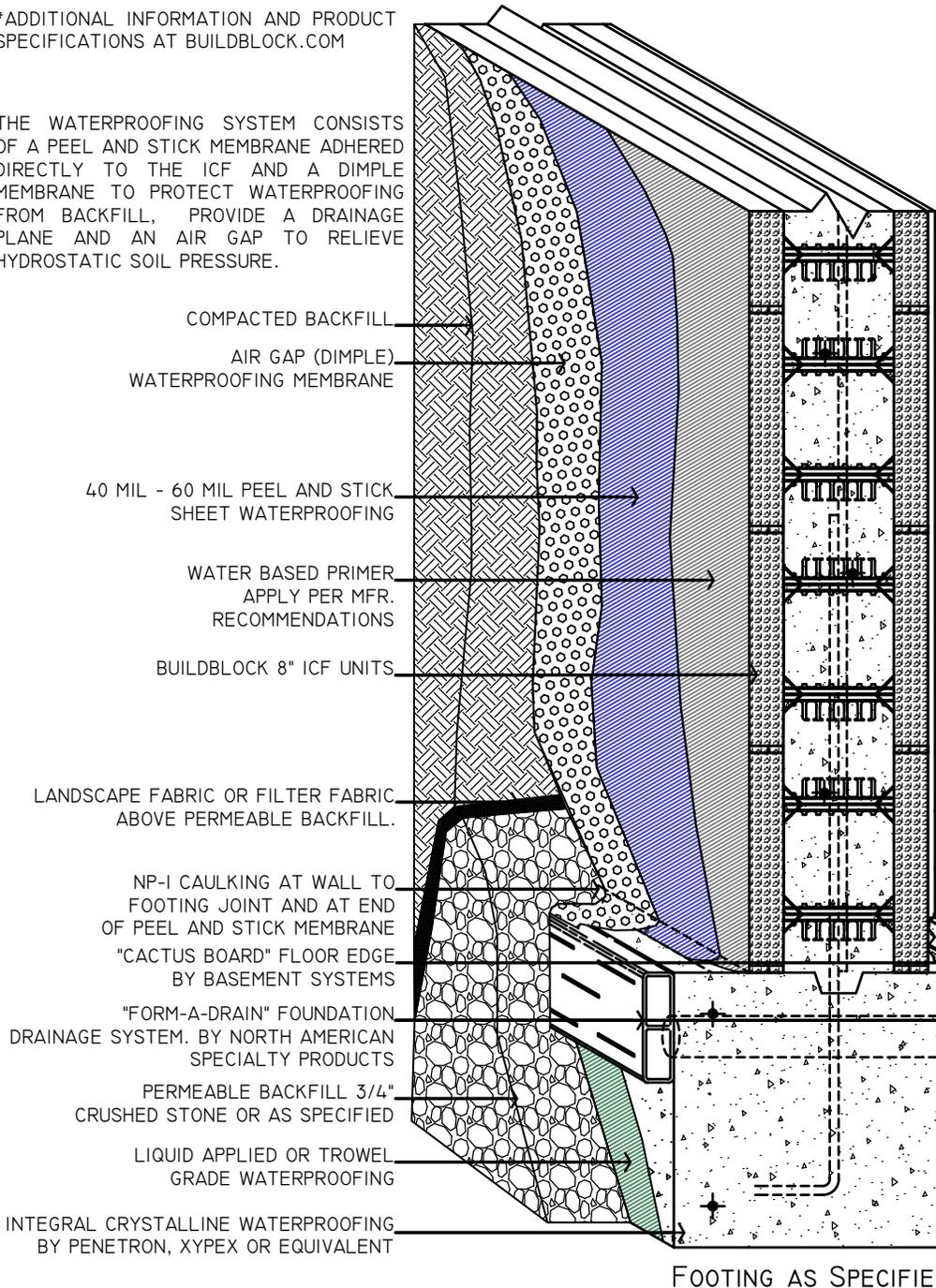
INSTALL WATERPROOFING BY MECHANICALLY ATTACHING A THIN FURRING STRIP OF PLASTIC OR METAL 6" - 12" ABOVE GRADE. IT IS ALSO POSSIBLE TO USE BASKET SCREWS SPACED 12" O.C. MAXIMUM. THIS ENSURES THE ADHESIVE HAS ADEQUATE TIME TO BOND TO THE FOAM OR PRIMER. THIS IS CRITICAL IN COLD AND HOT WEATHER OR WHEN SIGNIFICANT TEMPERATURE CHANGES OCCUR, SUCH AS DAYTIME HEATING AND OVERNIGHT COOLING.
